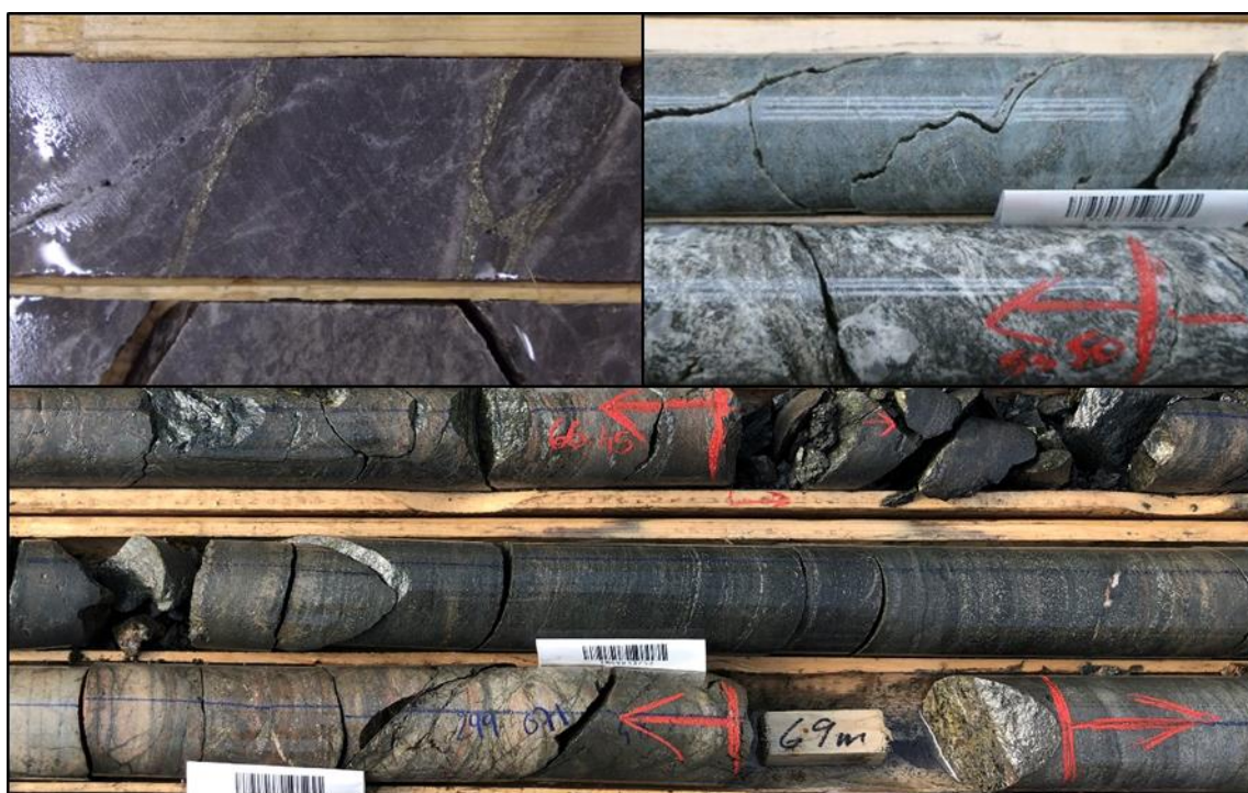
Clockwise from top-left corner: Pyrite as fracture fillings in hole NE-18-75, as fine disseminations in NE-17-54, and as disseminations and semi-massive beds in NE-19-124.
